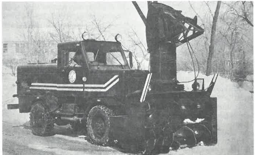
The Village snowblower is shown above. This piece of equipment picks up piles of snow in the business district. Glenview has a total of 35 vehicles equipped for snow removal.
