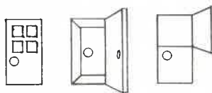
Wood & Glass Door with Vestibule Dutch Door
